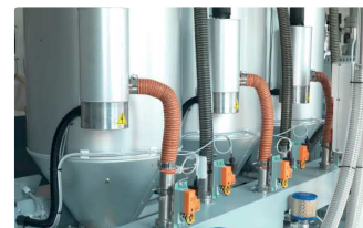
Modulating valve for airflow management.
